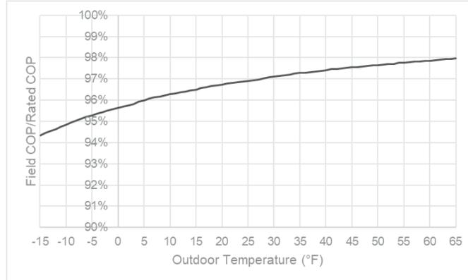
**Figure 5. Ratio of Field COP to Rated COP.**
