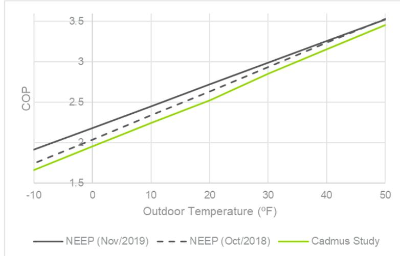
**Figure 3. COP Curves Based on NEEP Product Lists and on the Cadmus Study.<sup>6</sup>**
