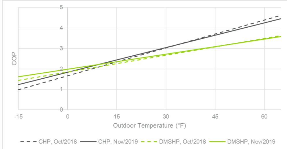
**Figure 2. Estimated COP as a Function of Outdoor Temperature, Based on NEEP ccASHP Product List Data**
