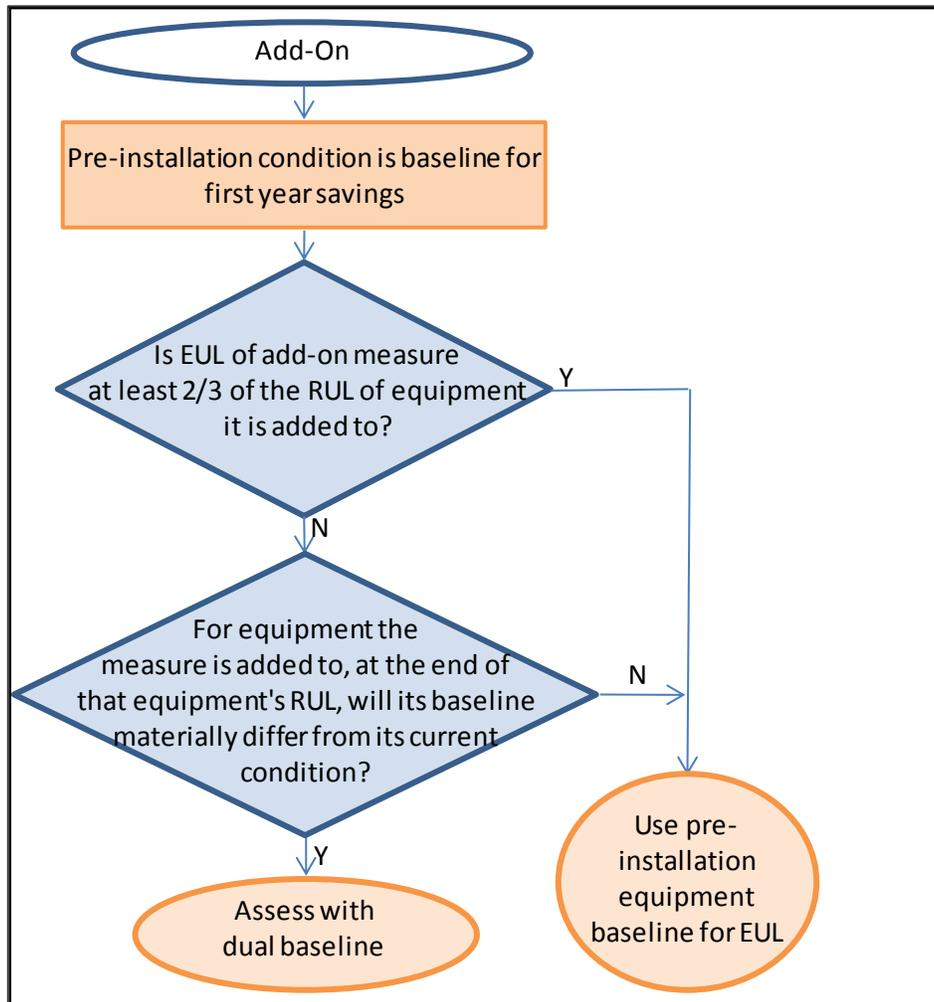
As shown in the figure, the evaluator must consider whether the system that receives the add-on measure has less of a remaining life than the add-on measure has full life, and if that will have a material effect on lifetime savings. The issue is most relevant for controls-related add-on measures. If the energy use of the equipment that is being controlled will predictably decline in the future for reasons unrelated to the add-on measure, then the lifetime savings should be adjusted accordingly.
