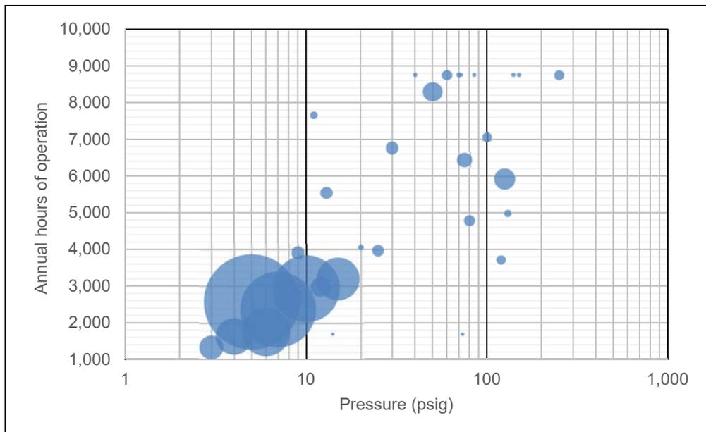
The means of comparison is slightly different in Figure 4 since two values (instead of one) are being compared. If there was an apparent relationship between pressure and leak factor, one would expect the two series to bunch up on opposite ends of the x-axis rather than what is currently observed.
