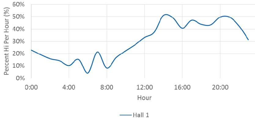
Since the bi-level lighting was occupancy controlled, it was not surprising that the light was at the high setting most frequently from 12:00 p.m. to 9:00 p.m. and on the low setting most frequently from 12:00 a.m. to 8:00 a.m.
